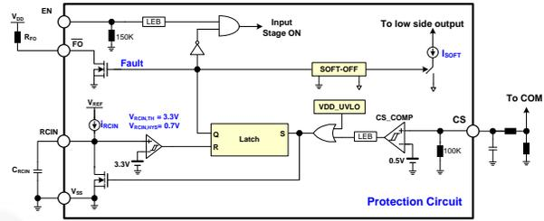
**Figure 43. Over-Current Protection**
