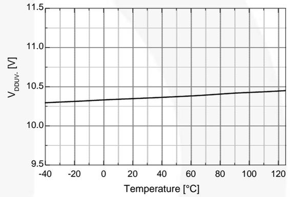
Figure 20.  $V_{DD}$  UVLO- vs. Temperature
