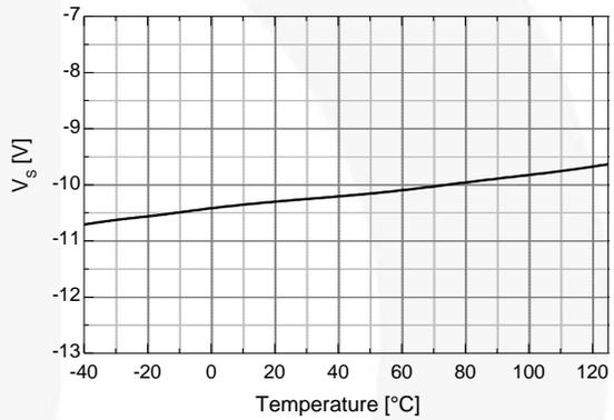
**Figure 14. Allowable Negative  $V_s$  Voltage vs. Temperature**
