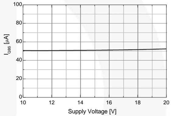
Figure 32. Quiescent  $V_{BS}$  Supply Current vs. Supply Voltage
