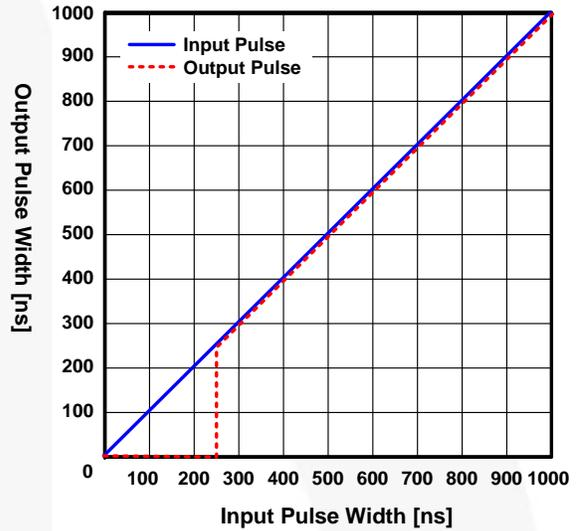
**Figure 47. Input Filter Characteristic of Narrow ON**
