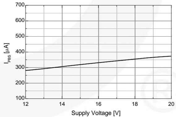
Figure 34. Operating  $V_{BS}$  Supply Current vs. Supply Voltage
