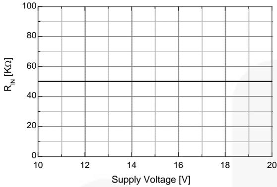
Figure 29. Input Pull-Down Resistance vs. Supply Voltage
