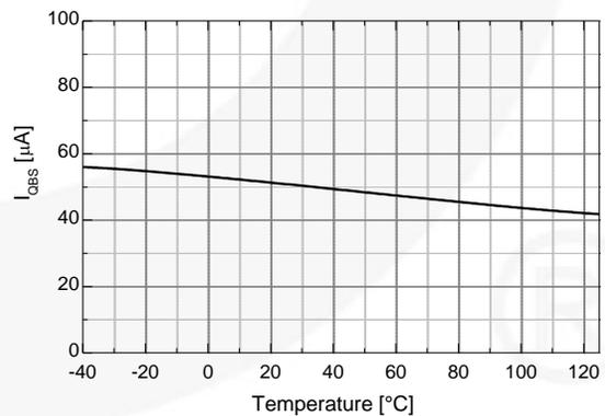
**Figure 16. Quiescent  $V_{BS}$  Supply Current vs. Temperature**
