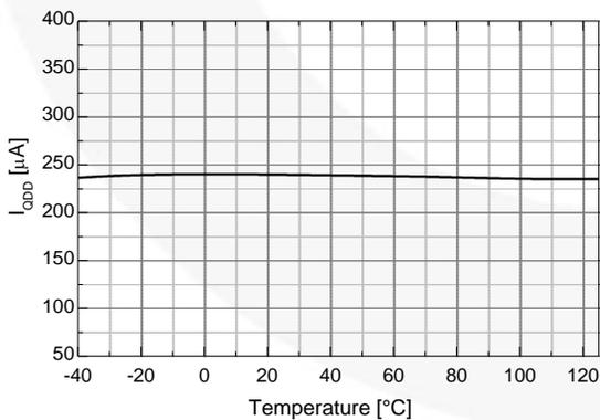
**Figure 15. Quiescent  $V_{DD}$  Supply Current vs. Temperature**
