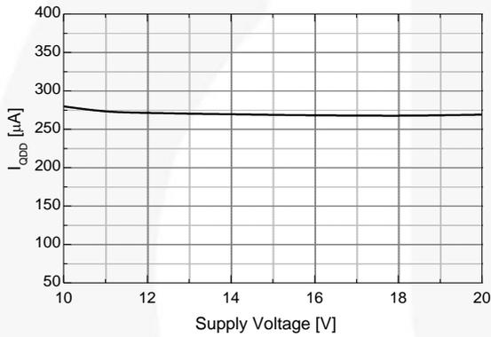
Figure 31. Quiescent  $V_{DD}$  Supply Current vs. Supply Voltage
