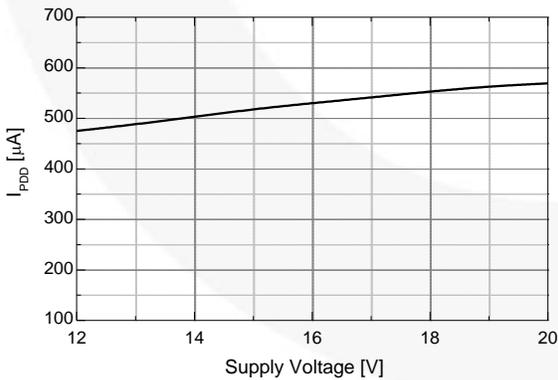
Figure 33. Operating  $V_{DD}$  Supply Current vs. Supply Voltage
