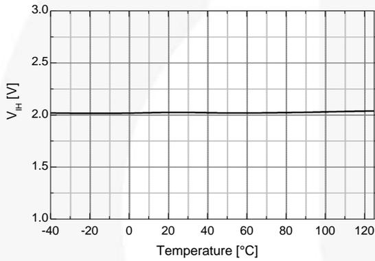
Figure 25. Logic HIGH Input Voltage vs. Temperature
