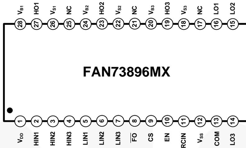
Figure 4. Pin Assignments
