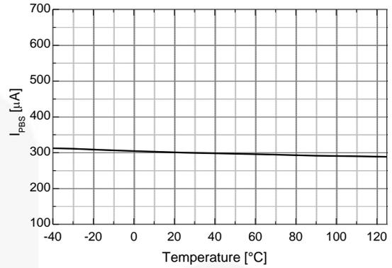
Figure 18. Operating  $V_{BS}$  Supply Current vs. Temperature
