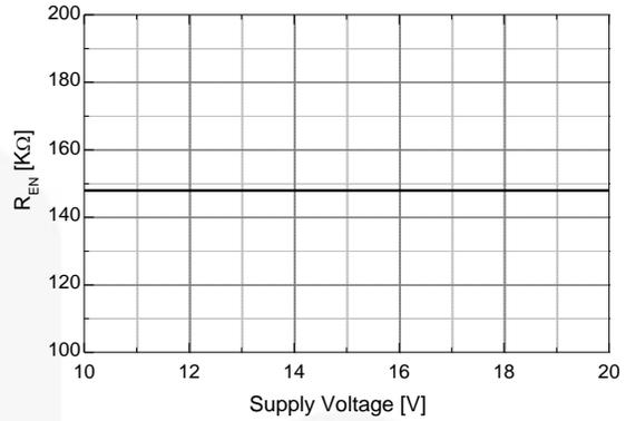
Figure 30. Enable Pin Pull-Down Resistance vs. Supply Voltage
