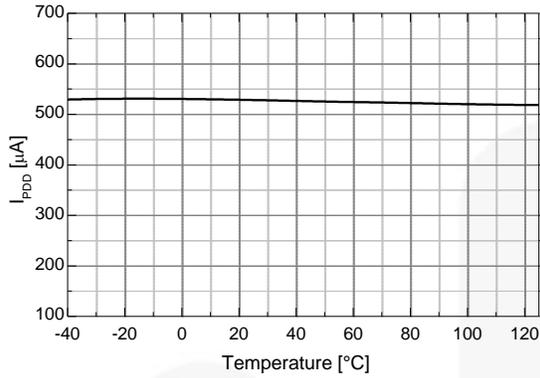
Figure 17. Operating  $V_{DD}$  Supply Current vs. Temperature
