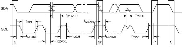
Figure 41. I<sup>2</sup>C Bus AC Timing Diagram
