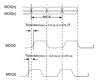
Figure 4. Timing Diagram for tDDKHMH
