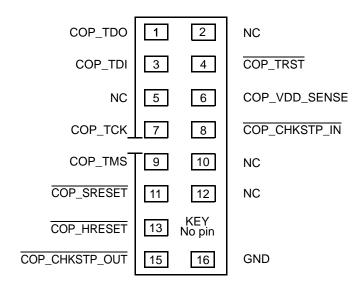
Figure 65. COP Connector Physical Pinout
