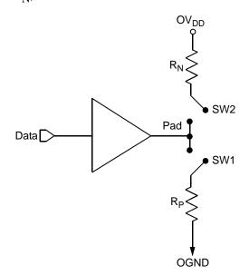
Figure 64. Driver Impedance Measurement
