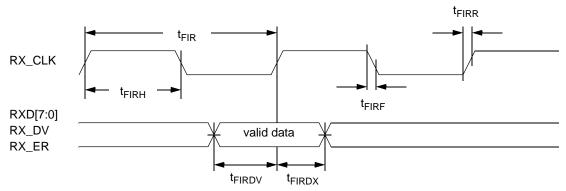
Figure 8. FIFO Receive AC Timing Diagram
