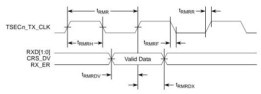
Figure 21. RMII Receive AC Timing Diagram
