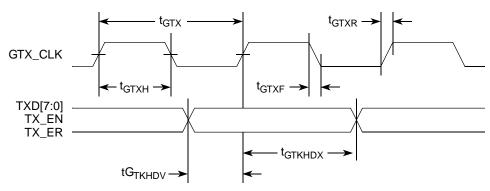
Figure 9. GMII Transmit AC Timing Diagram
