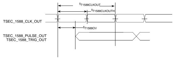
Figure 26. eTSEC IEEE 1588 Output AC Timing
