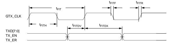
Figure 7. FIFO Transmit AC Timing Diagram
