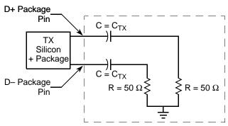
Figure 57. Compliance Test/Measurement Load
