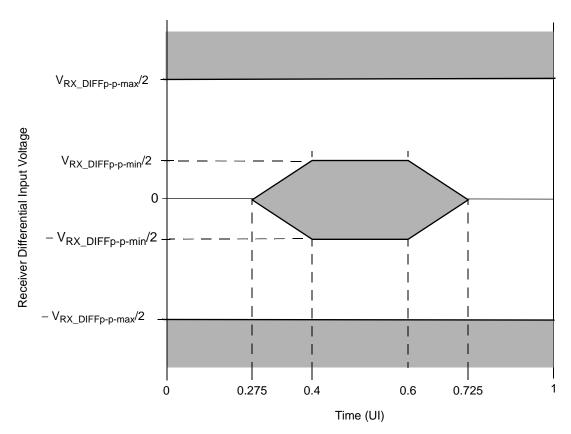
Figure 24. SGMII Receiver Input Compliance Mask
