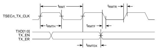
Figure 19. RMII Transmit AC Timing Diagram
