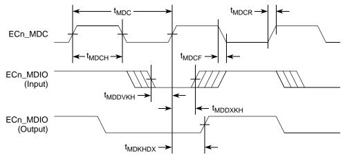
Figure 28. MII Management Interface Timing Diagram
