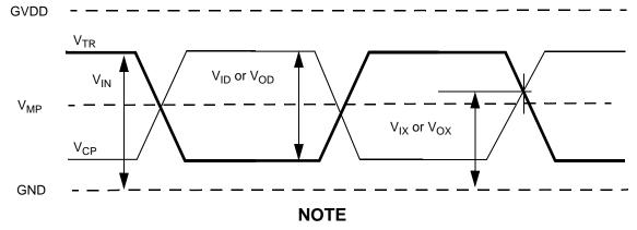
VID specifies the input differential voltage |VTR - VCP| required for switching, where VTR is the true input signal (such as  $\overline{MCK}$  or  $\overline{MDQS}$ ) and VCP is the complementary input signal (such as  $\overline{MCK}$  or  $\overline{MDQS}$ ).
