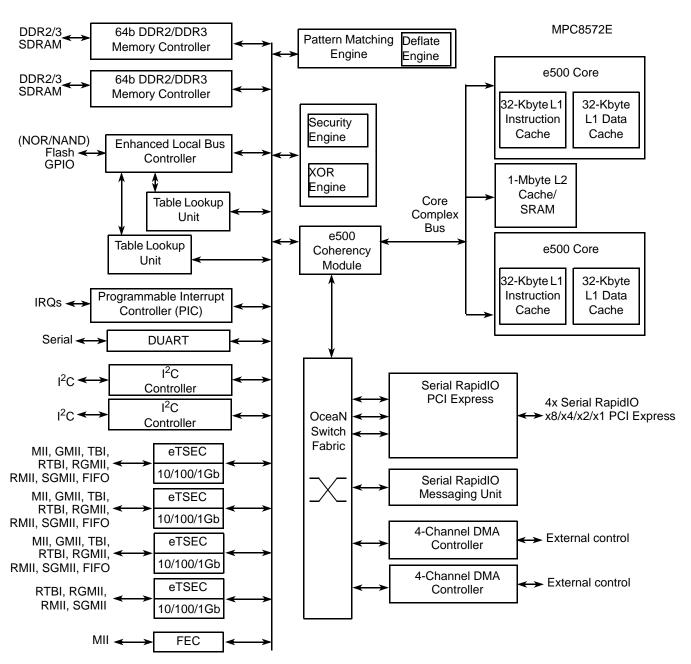
Figure 1. MPC8572E Block Diagram
