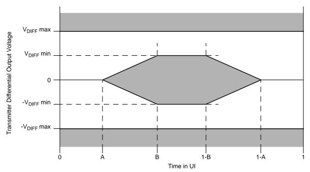
Figure 58. Transmitter Output Compliance Mask
