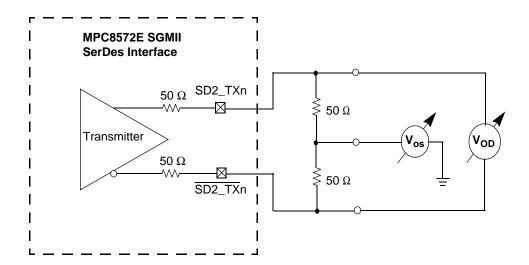
Figure 23. SGMII Transmitter DC Measurement Circuit
