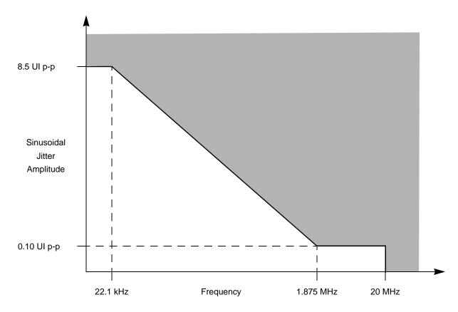
Figure 59. Single Frequency Sinusoidal Jitter Limits
