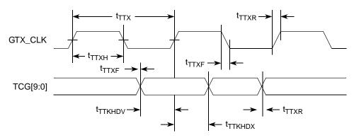
Figure 15. TBI Transmit AC Timing Diagram
