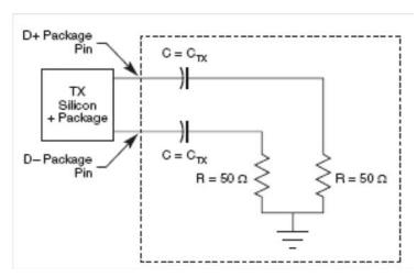
Figure 25. SGMII AC Test/Measurement Load
