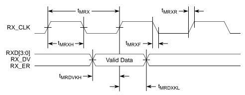
Figure 14. MII Receive AC Timing Diagram
