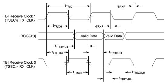
Figure 16. TBI Receive AC Timing Diagram
