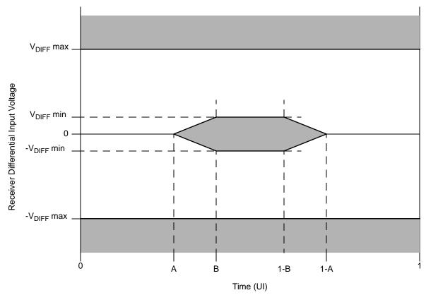
Figure 60. Receiver Input Compliance Mask
