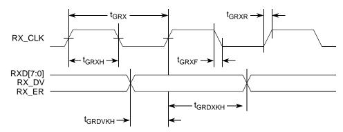
Figure 11. GMII Receive AC Timing Diagram
