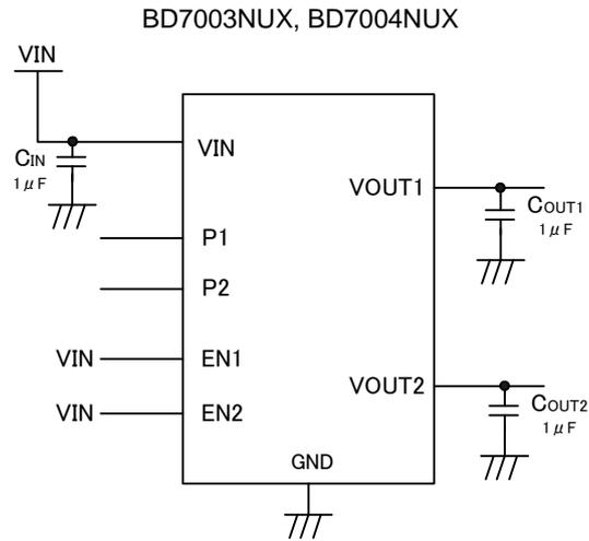
Figure2. Application Circuit
