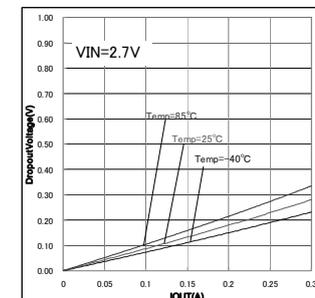
Fig.24. Drop Out Voltage
