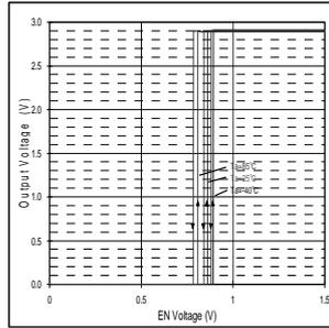
Fig.17. EN2 Threshold
