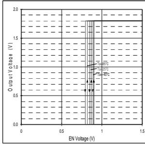
Fig.16. EN1 Threshold
