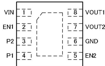
Note : Recommend connecting the Thermal Pad to the GND for excellent power dissipation.
