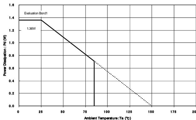
Fig.1. VSON008X2020 Power dissipation heat reduction characteristics (Reference)
