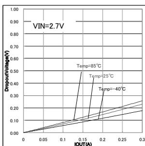
Fig.25. Drop Out Voltage
