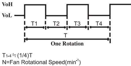
**Figure 5 FG Signal Output Circuit: Open Collector**
