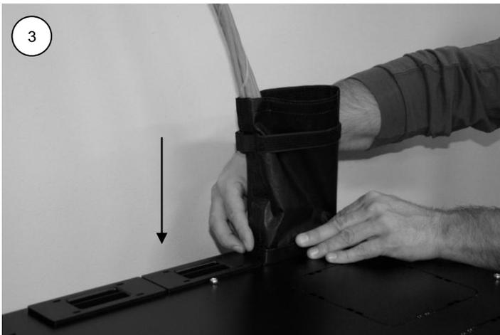
Step 3: Reattach the hook and loop side strip and the cinch tie. Align Cool Boot fitting with the cabinet top bezel and insert by pressing down on the top of the outer edges of the fitting assembly.
