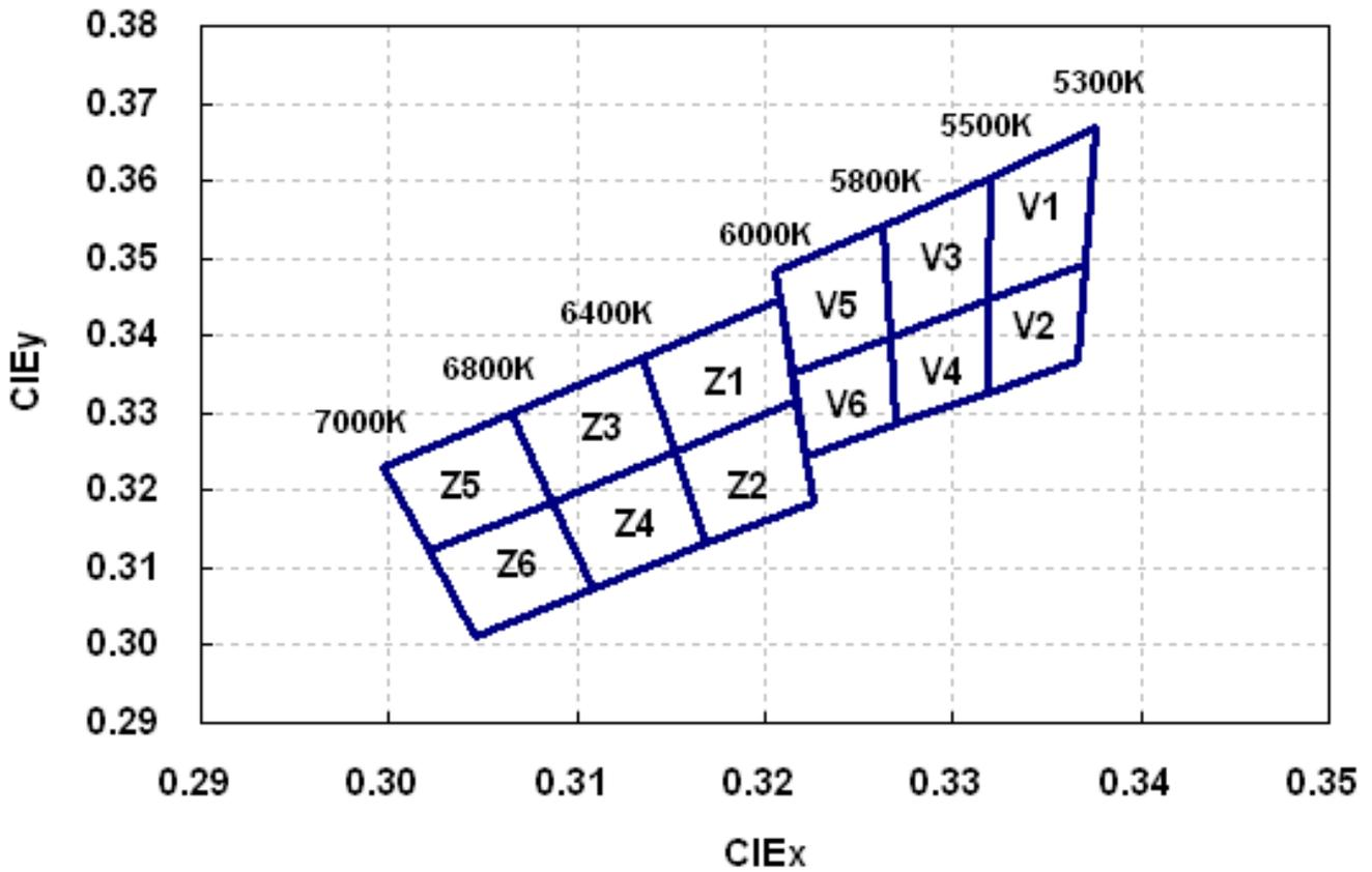
Tolerance on each Hue (x, y) bin is +/- 0.01.
