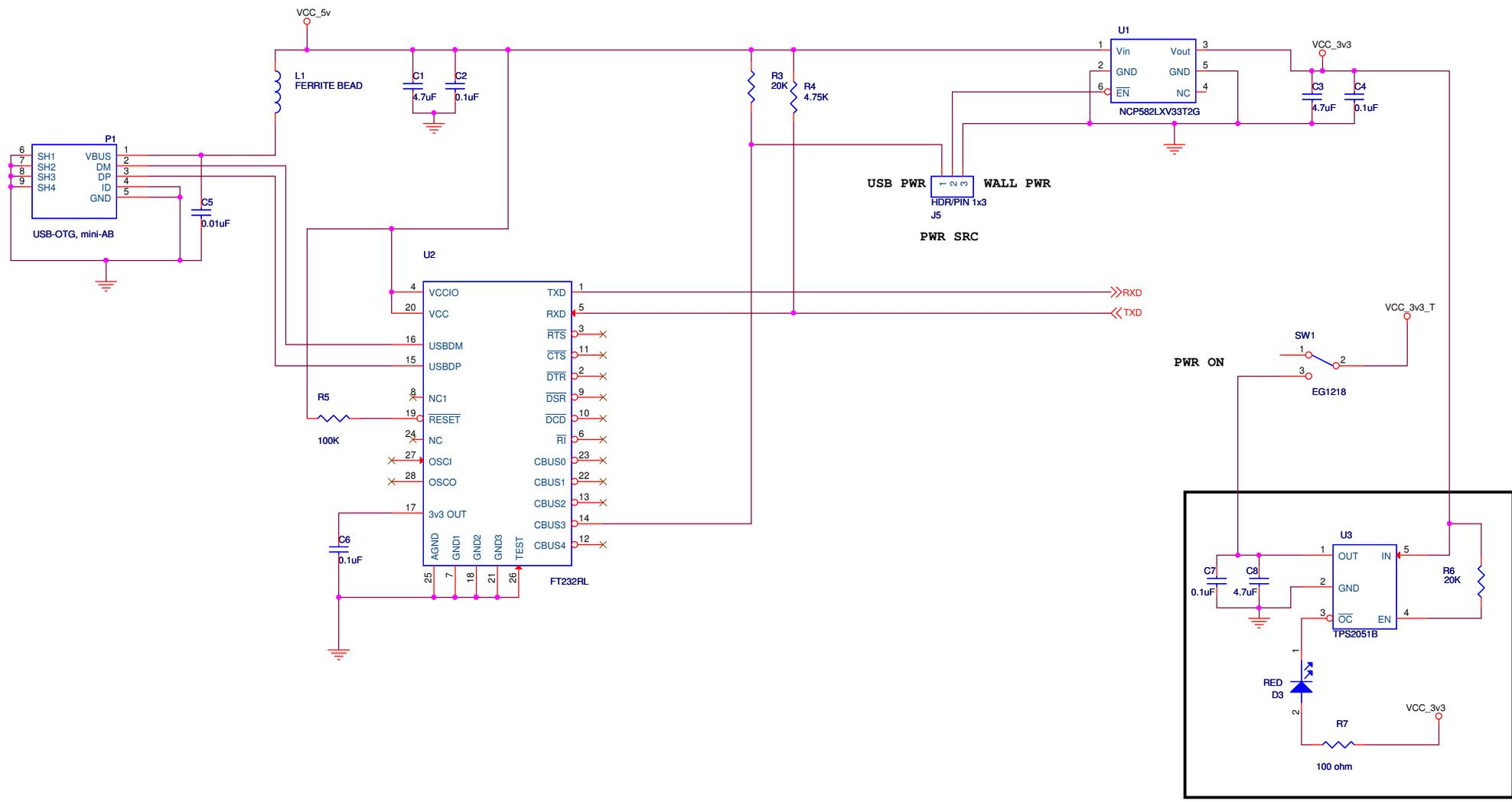
Figure 18. ZMOTION 20-Pin Development Board Schematic Diagram, #2 of 2
