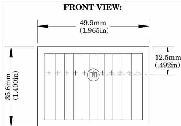
**Figure 9. Flat Lens: AA 0.9 GI T1**
