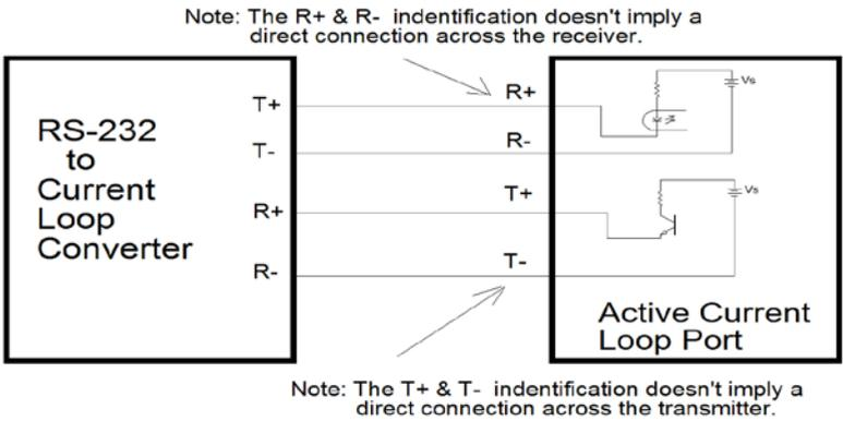
Figure 2. Connection to an Active Current Loop
