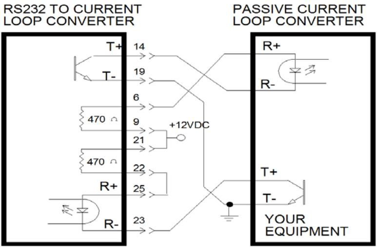
Figure 3. Connection to a Passive Current Loop
