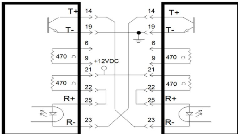
Figure 4. Interconnection of Two Current Loop converters
