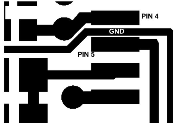
FIGURE 15. LAYOUT DETAIL OF GND BETWEEN PINS 4 AND 5
