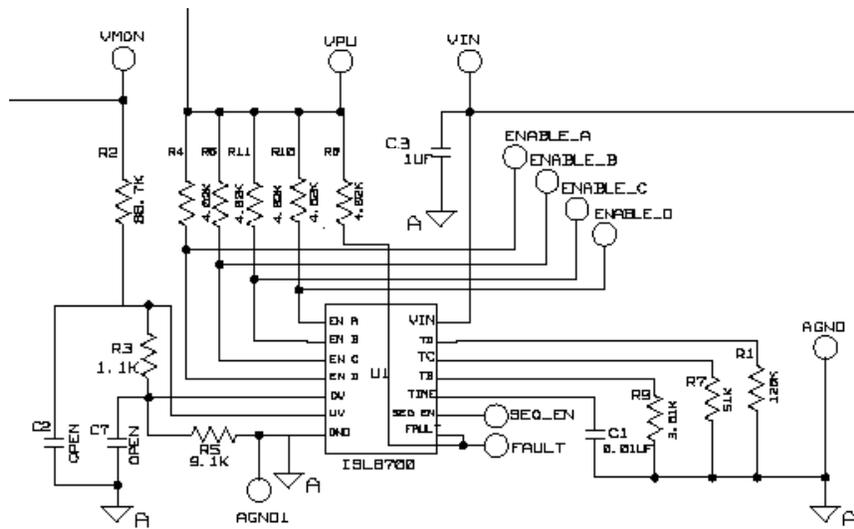
FIGURE 16. ISL870XAEVAL1 PHOTOGRAPH AND SCHEMATIC OF LEFT CHANNEL
