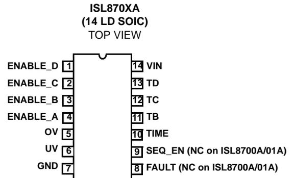
ISL8701A, ISL8703A, ISL8705A PINS 1-4 ARE ENABLE# FUNCTION
