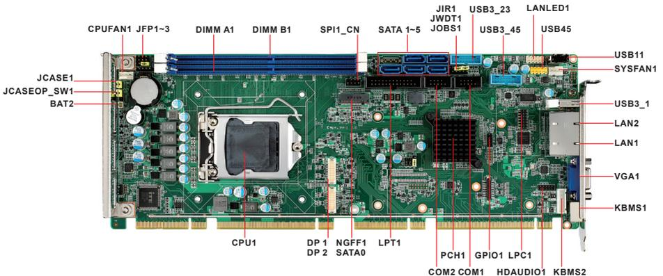
**Figure 1: Board Layout: Jumper and Connector Locations**
