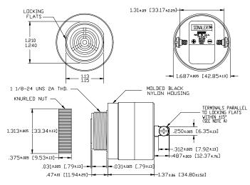
NOTE AF TERMINALS-032 BRASS TIN PLATED, TAPPED FOR #6-32 SCREW. TWO #6-32 NICKEL PLATED BRASS SCREWS INCLUDED. WILL ACCEPT 1/4' QUICK CONNECT. NOTE B: MOUNTING- REMOVE BLACK PLASTIC NUT AND INSERT THREADED FRONT THROUGH 1.25' HOLE PUNCHED IN PANEL, IF DRIENTATION IS NEEDED, NOTE LOCKING FLATS ON DRAVING. SCREW NUT BACK ON. DO NOT OVERTIGHTEN.
