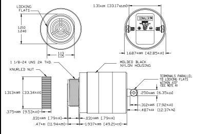
NOTE AF TERMINALS-032 BRASS TIN PLATED, TAPPED FOR #6-32 SCREW. TWO #6-32 NICKEL PLATED BRASS SCREWS INCLUBED. WILL ACCEPT 1/4' QUICK CONNECT. NOTE B: MOUNTING- REMOVE BLACK PLASTIC NUT AND INSERT THREADED FRONT THROUGH 1.25' HOLE PUNCHED IN PANEL, IF DRIENTATION IS NEEDED, NOTE LOCKING FLATS ON DRAWING. SCREW NUT BACK ON. DO NOT OVERTIGHTEN.
