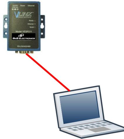
Figure 11. Console Mode Setup
