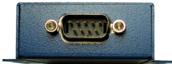
Figure 5. DB-9M Serial Port Connector
