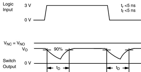
Figure 2. Break-Before-Make Interval
