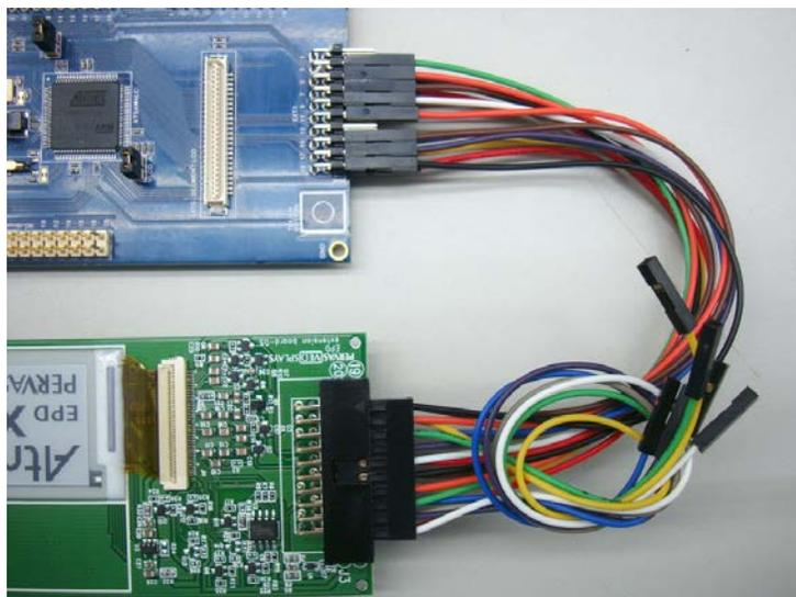
Connect the EPD Extension board to Atmel SAM4L Xplained Pro header marked as **EXT3** via the 20 pins cable.
