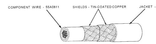
JACKET - RADIATION-CROSSLINKED. MODIFIED ETFE
