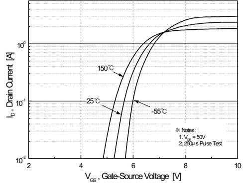
Figure 2. Transfer Characteristics
