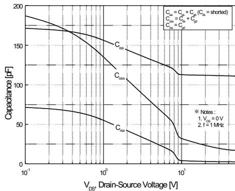
Figure 5. Capacitance Characteristics
