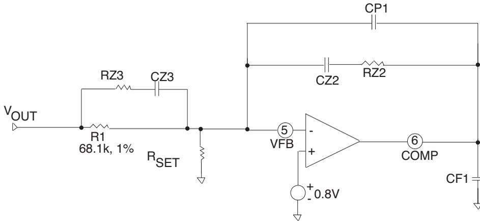
$$R_{SET} = 54.48 / (V_{OUT} - 0.8V) (k\Omega)$$
