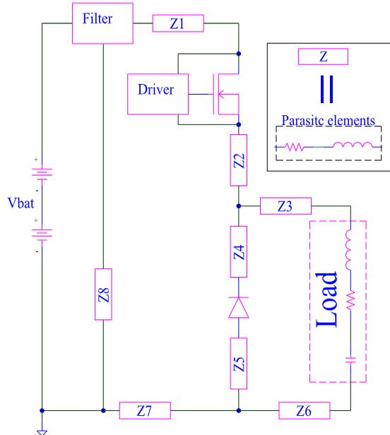
**Figure 7: typical schematic of a power module**
