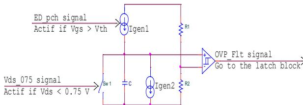
Time to charge the capacitor and latch a fault ( $I_{gen1} + C$ ) = 9 $\mu$ s
