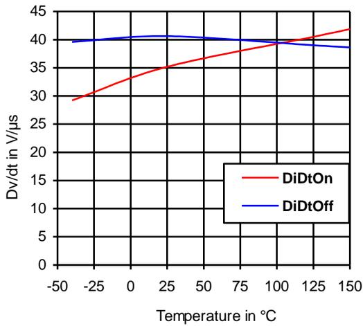
**Figure 16: Dv/dt on & off vs. temperature**
