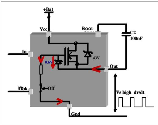
The IR3330S has a high  $dv/dt$  immunity system. This function creates a negative gate biasing if the output voltage exceed 1.7V. So this device can be implemented in an H-bridge configuration.
