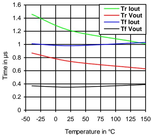
**Figure 14: Rise and fall time vs. temperature**
