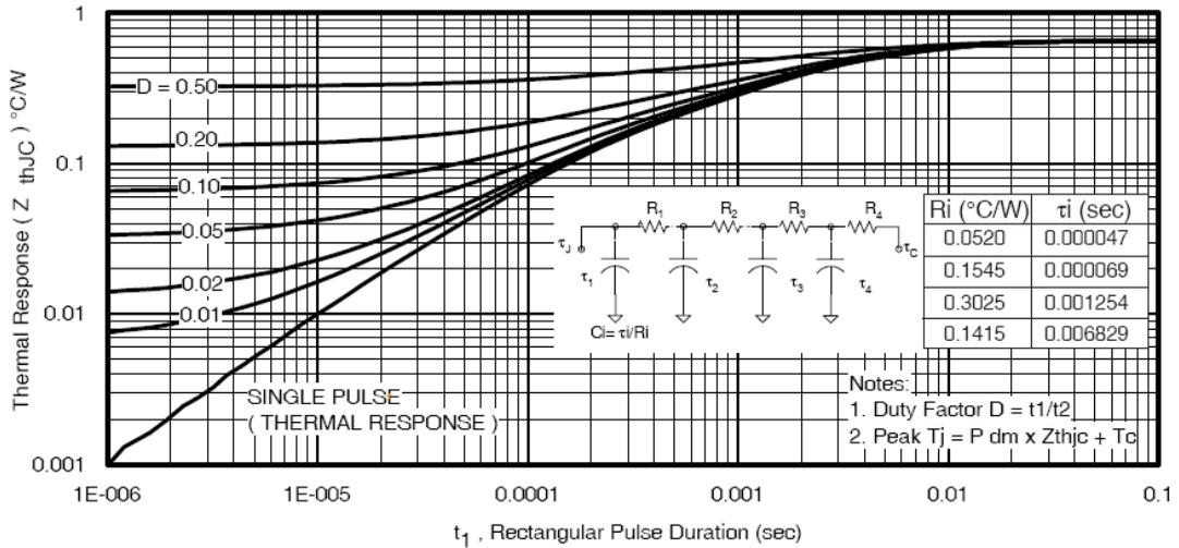
**Figure 15: Transient thermal impedance and model vs. time**
