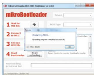
Click OK button after the uploading process is finished. Press Reset button on mikromedia plus for FT90x board and wait for 5 seconds. Your program will run automatically.
