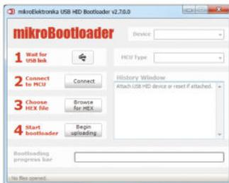
To start, connect the USB cable, or if already connected press the Reset button on your mikromedia plus for FT90x. Click the Connect button within 5s to enter the bootloader mode, otherwise existing microcontroller program will execute.
