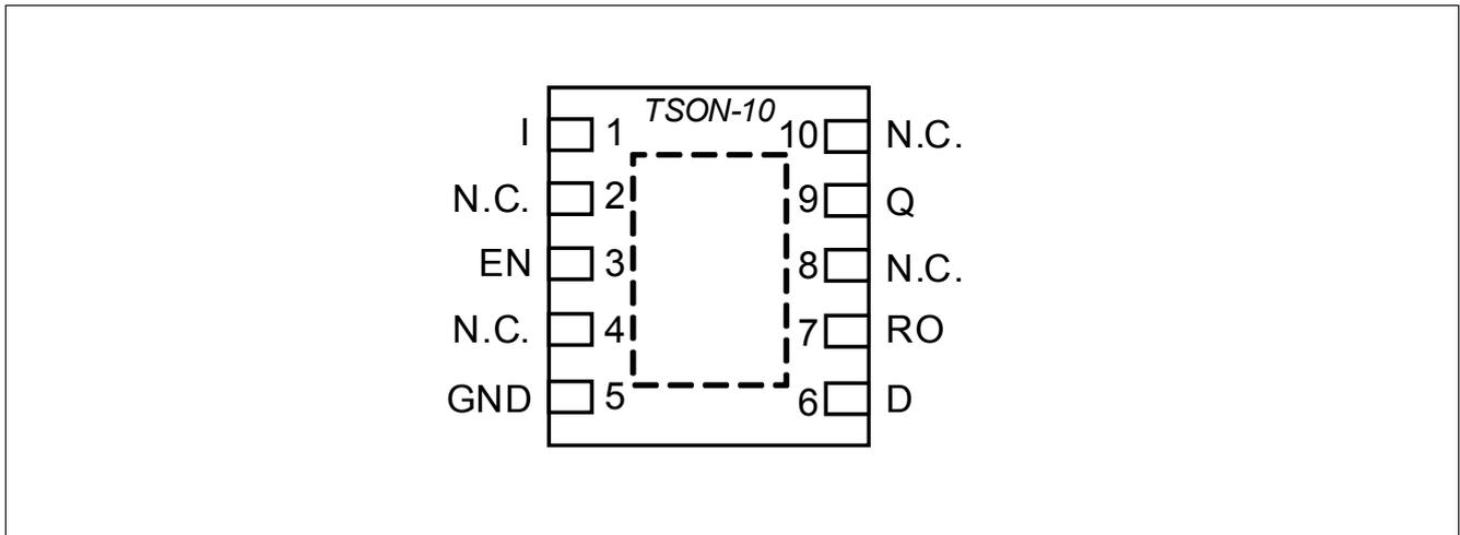
Figure 3 Pin Configuration TLS805D1 in PG-TSON-10 package
