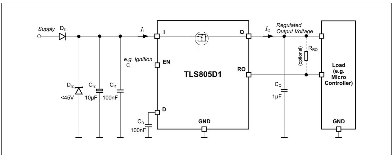
Figure 7 Application Diagram
