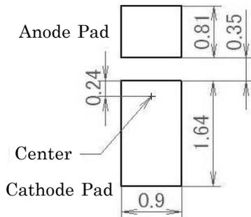
Mountability and solderability need to be optimized with actual conditions such as amount of solder, reflow temperature applied in the process.
