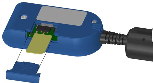
2. Insert the SIM card into the card holder with the gold contact side facing down as shown.
