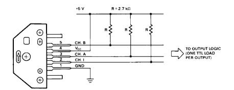
Figure 1. Pull-up Resistors on HEDS-9X40 Encoder Module Outputs.
