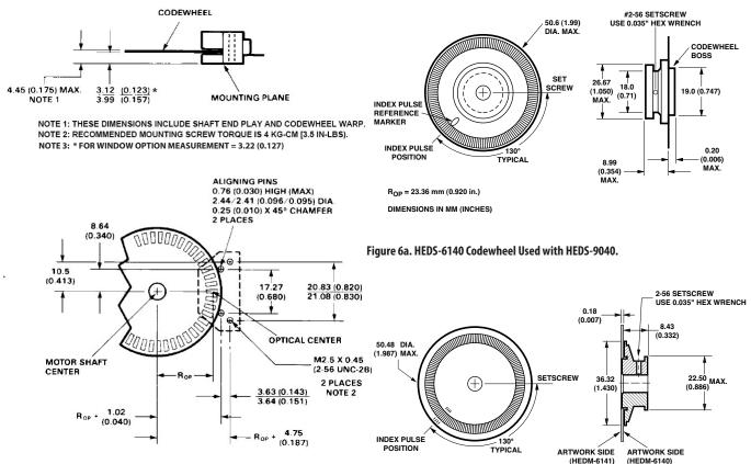
Figure 5. Mounting Plane Side A.
