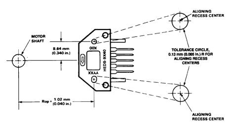
Figure 2. HEDS-9X40 Mounting Tolerance.
