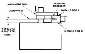
NOTE 1: THIS DIMENSION IS FROM THE MOUNTING PLANE TO THE NON-HUB SIDE OF THE CODEWHEEL.
