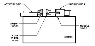
Figure 3. Alignment Tool is Used to Set Height of Codewheel.
