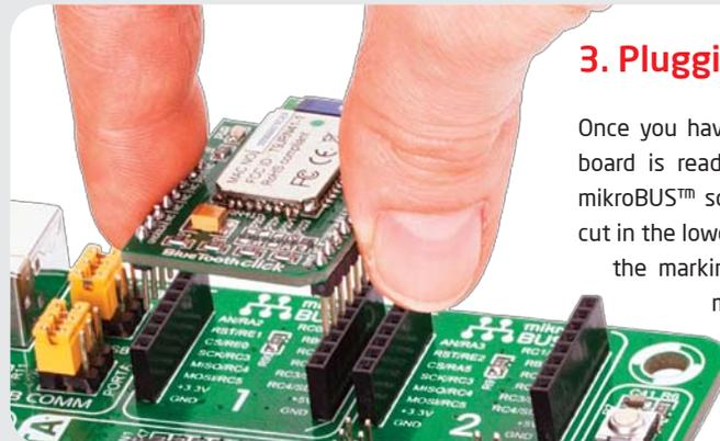
Once you have soldered the headers your board is ready to be placed into desired mikroBUS™ socket. Make sure to align the cut in the lower-right part of the board with the markings on the silkscreen at the mikroBUS™ socket. If all the pins are aligned correctly, push the board all the way into the socket.
