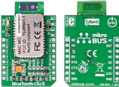
BLUETOOTH click is an accessory board in **mikroBus™** form factor. It features **RN-41** fully qualified Bluetooth 2.1/2.0/1.2/1.1 module with UART interface which is easy and simple to use. Device is a Class 1 high power radio and can operate up to **100m distance**. Board offers low power (30mA connected, less than 10mA sniffmode), highly economic Bluetooth radio for adding wireless capability to your products. Board is designed to use 3.3V power supply only.
