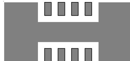
(e) Copper Area =  $70 \text{ mm}^2$ ,  $\theta_{JA} = 49^\circ\text{C/W}$
