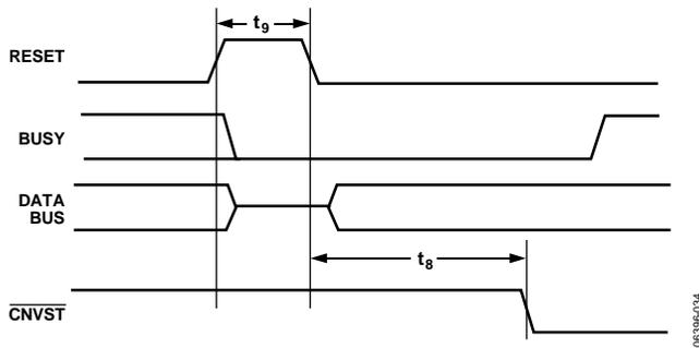
Figure 34. RESET Timing
