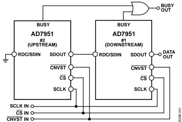
Figure 41. Two AD7951 Devices in a Daisy-Chain Configuration
