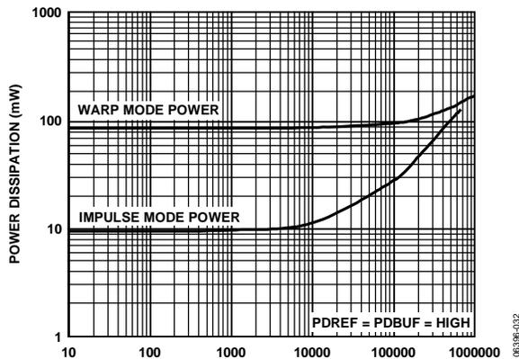
Figure 32. Power Dissipation vs. Sample Rate
