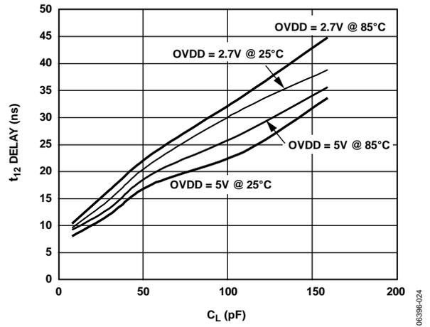
Figure 24. Typical Delay vs. Load Capacitance C<sub>L</sub>
