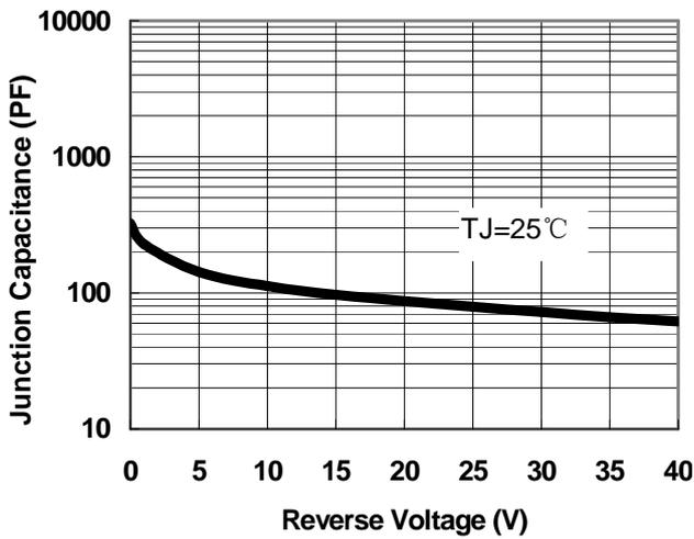
Fig.1-Typical Junction Capacitance
