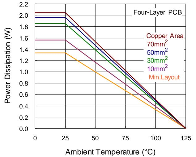
Figure 7. Derating Curves for RT8292B Package
