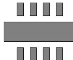
(c) Copper Area = 30mm<sup>2</sup>,  $\theta_{JA} = 54^\circ\text{C/W}$
