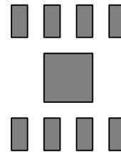
(a) Copper Area = (2.3 x 2.3) mm<sup>2</sup>,  $\theta_{JA} = 75^\circ\text{C/W}$
