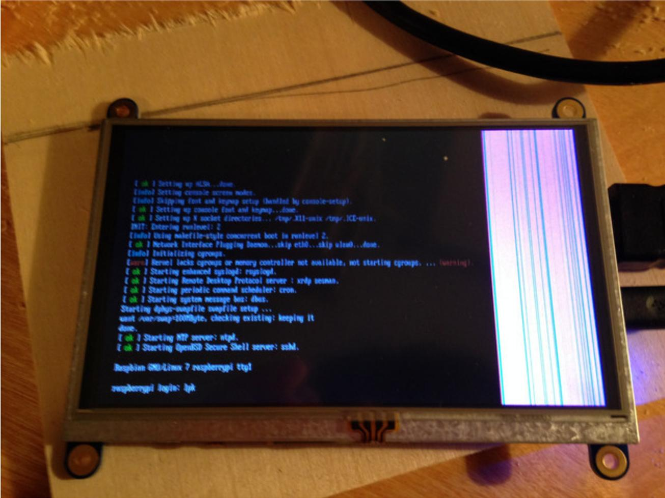
**It is not broken** - what is happening is you are sending 640x480 data to the monitor but since it does not have a scaler, and the display is 800x480, the remaining 160 pixels are
