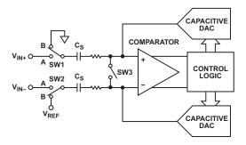
Figure 63. ADC Conversion Phase
