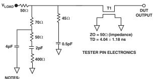
THE WORST CASE TRANSMISSION LINE DELAY IS SHOWN AND CAN BE USED FOR THE OUTPUT TIMING ANALYSIS TO REFELECT THE TRANSMISSION LINE EFFECT AND MUST BE CONSIDERED. THE TRANSMISSION LINE (TD), IS FOR LOAD ONLY AND DOES NOT AFFECT THE DATA SHEET TIMING SPECIFICATIONS.
