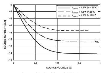
Figure 40. Driver Type D Current (1.8  $VV_{DDEXT}$ )
