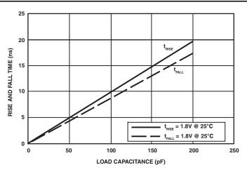
Figure 47. Driver Type C Typical Rise and Fall Times (10%–90%) vs. Load Capacitance (1.8 V V<sub>DDEXT</sub>)
