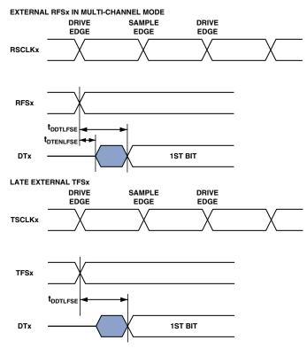
Figure 22. Serial Ports — External Late Frame Sync
