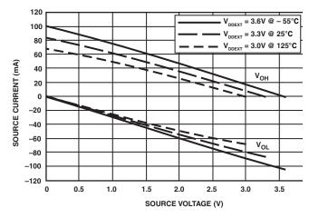
Figure 35. Driver Type C Current (3.3 V V<sub>DDEXT</sub>)
