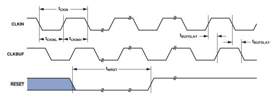
Figure 10. Clock and Reset Timing
