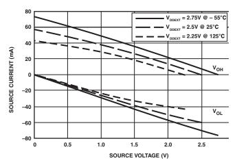
Figure 36. Drive Type C Current (2.5 V V<sub>DDEXT</sub>)
