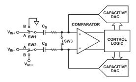
Figure 62. ADC Acquisition Phase
