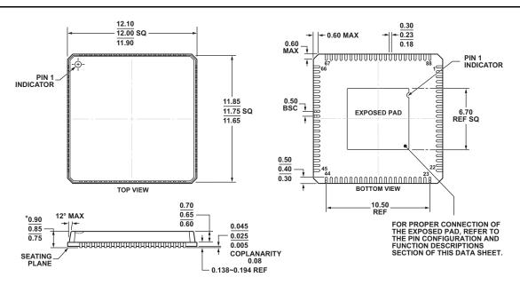
\*COMPLIANT TO JEDEC STANDARDS MO-220-VRRD EXCEPT FOR MINIMUM THICKNESS AND LEAD COUNT.
