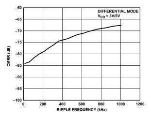
Figure 61. CMRR vs. Common-Mode Ripple Frequency
