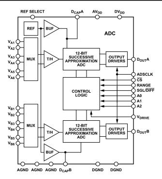
Figure 8. ADC (Internal) Functional Block Diagram
