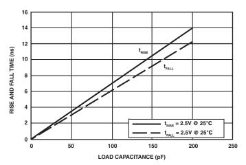
Figure 48. Driver Type C Typical Rise and Fall Times (10%–90%) vs. Load Capacitance (2.5 V V<sub>DDEXT</sub>)
