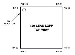
Figure 89. 120-Lead LQFP Package Lead Configuration (Top View)
