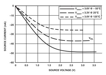
Figure 38. Driver Type D Current (3.3 V V<sub>DDEXT</sub>)
