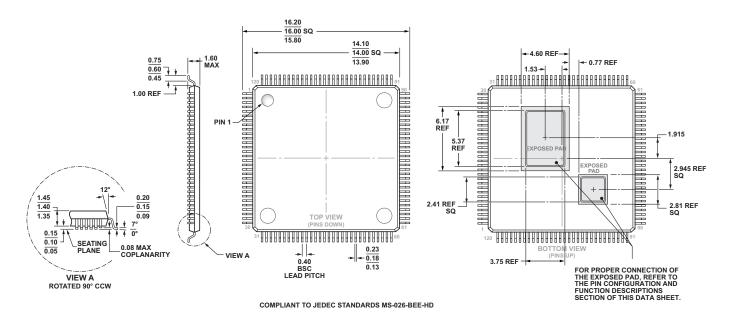
Figure 93. 120-Lead Low Profile Quad Flat Package, Exposed Pad [LQFP\_EP]<sup>1</sup> (SW-120-2)
