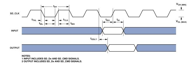
Figure 18. RSI Controller Timing
