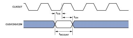
Figure 28. Up/Down Counter/Rotary Encoder Timing
