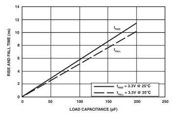
Figure 49. Driver Type C Typical Rise and Fall Times (10%–90%) vs. Load Capacitance (3.3 V V<sub>DDEXT</sub>)
