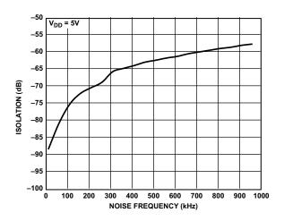
Figure 51. Channel-to-Channel Isolation
