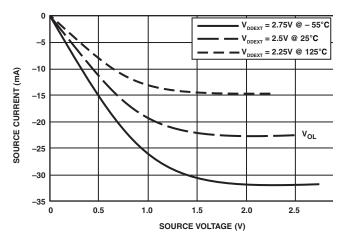
Figure 39. Driver Type D Current (2.5 V V<sub>DDEXT</sub>)
