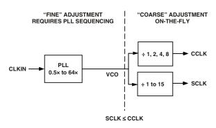
Figure 5. Frequency Modification Methods
