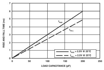
Figure 45. Driver Type B Typical Rise and Fall Times (10%–90%) vs. Load Capacitance (2.5 V V<sub>DDEXT</sub>)
