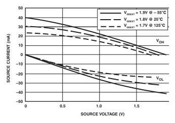
Figure 37. Driver Type C Current (1.8 V V<sub>DDEXT</sub>)
