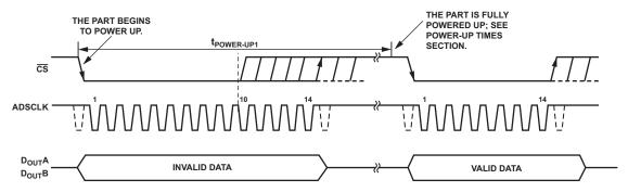
Figure 82. Exiting Partial Power-Down Mode
