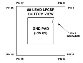
Figure 92. 88-Lead LFCSP Lead Configuration (Bottom View)
