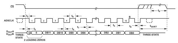
Figure 87. Serial Interface Timing Diagram
