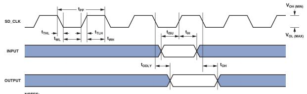
NOTES: 1 INPUT INCLUDES SD\_Dx AND SD\_CMD SIGNALS. 2 OUTPUT INCLUDES SD\_Dx AND SD\_CMD SIGNALS.
