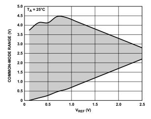
Figure 71. Input Common-Mode Range vs.  $V_{REF}$  (2 ×  $V_{REF}$  Range,  $V_{DD}$  = 5 V)
