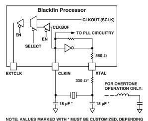
NOTE: VALUES MARKED WITH \* MUST BE CUSTOMIZED, DEPENDING ON THE CRYSTAL AND LAYOUT. PLEASE ANALYZE CAREFULLY. FOR FREQUENCIES ABOVE 33 MHz, THE SUGGESTED CAPACITOR VALUE OF 18 pF SHOULD BE TREATED AS A MAXIMUM, AND THE SUGGESTED RESISTOR VALUE SHOULD BE REDUCED TO 0  $\Omega$ .
