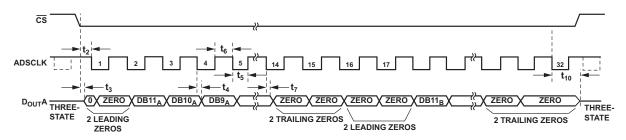
Figure 88. Reading Data from Both ADCs on One  $D_{\rm OUT}$  Line with 32 ADSCLKs
