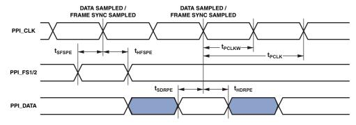
Figure 14. PPI GP Rx Mode with External Frame Sync Timing
