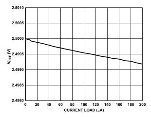
Figure 58. V<sub>REF</sub> vs. Reference Output Current Drive
