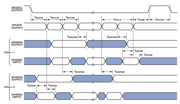
Figure 23. Serial Peripheral Interface (SPI) Port—Master Timing
