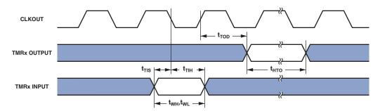
Figure 26. Timer Cycle Timing
