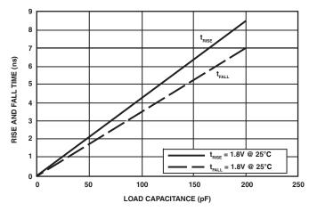
Figure 44. Driver Type B Typical Rise and Fall Times (10%–90%) vs. Load Capacitance (1.8 V V<sub>DDEXT</sub>)
