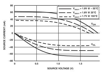
Figure 34. Driver Type B Current (1.8 V V<sub>DDEXT</sub>)
