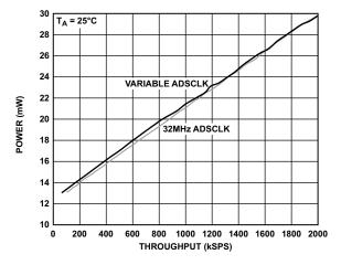
Figure 86. Power vs. Throughput in Normal Mode with  $V_{DD} = 5 V$
