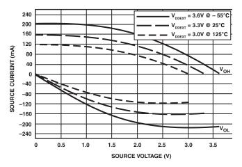
Figure 32. Driver Type B Current (3.3 V V<sub>DDEXT</sub>)
