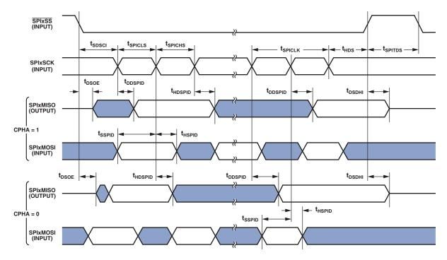
Figure 24. Serial Peripheral Interface (SPI) Port—Slave Timing
