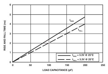
Figure 46. Driver Type B Typical Rise and Fall Times (10%–90%) vs. Load Capacitance (3.3 V  $V_{\rm DDEXT}$ )
