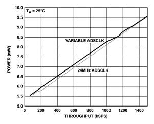
Figure 85. Power vs. Throughput in Normal Mode with  $V_{DD} = 3 V$
