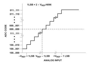
Figure 79. Twos Complement Transfer Characteristic with  $V_{\rm RFE} \pm V_{\rm RFE}$  Input Range
