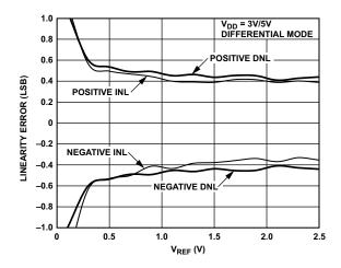
Figure 56. Linearity Error vs. V<sub>REF</sub>
