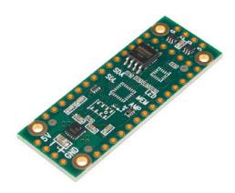
**Description:** This low-cost (LC) Teensy Prop Shield is meant for making light and sound effects on small, handheld props and wearable costumes. This shield features a 2W audio amp, high-speed 5V buffers for driving APA102 LEDs, and an 8MB flash memory. This economical board is approximately the size of a Teensy, just slightly longer to allow space for mounting holes and connections for power, speaker and LEDs.
