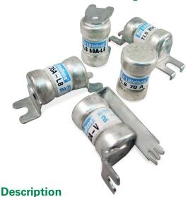
Littelfuse TLS Series fuses are designed specifically for the protection of telecommunications equipment. TLS fuses have been engineered to operate up to 170 Vdc to provide current-limiting short-circuit protection for cables and components found in the DC power distribution circuits of telecommunications systems. The compact design and multiple mounting configurations of the TLS series allow it to be used in a variety of applications.
