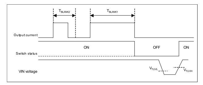
Figure 39. Over-current detection, shutdown operation (return with UVLO operation)
