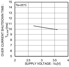
Figure 16. Over current shutdown time
