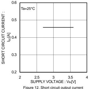
Figure 12. Short circuit output current (BD2202G)
