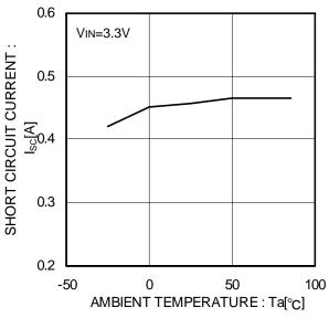
Figure 13. Short circuit output current (BD2202G)
