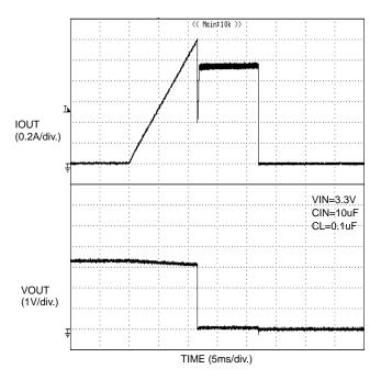
Figure 35. Current limit response Ramped load (1A/10ms) (BD2206G)
