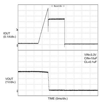
Figure 34. Current limit response Ramped load (1A/10ms) (BD2202G)
