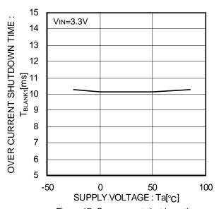
Figure 17. Over current shutdown time
