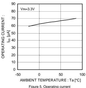
Figure 5. Operating current EN Enable
