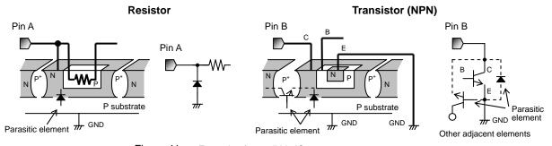
Figure 41. Example of monolithic IC structure
