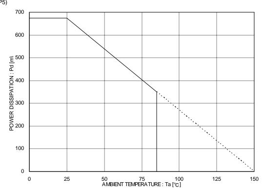
Figure 40. Power dissipation curve (Pd-Ta Curve)
