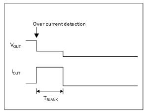
Figure 3. Over current limits characteristics
