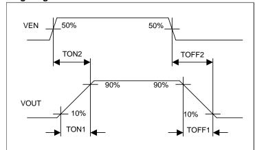
Figure 2. Switch Turn on / off time
