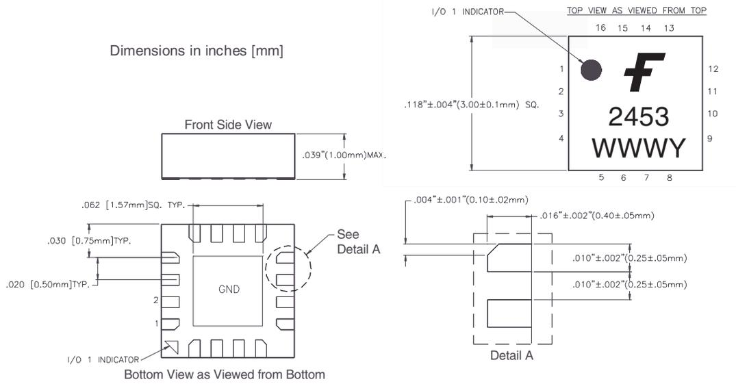
**Note:** Dimensions do not include protrusions or mold flash. These are not to exceed 0.006" (.155mm) on any side.
