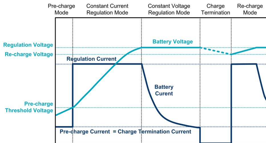
Figure 3. Battery Charger Operation Modes
