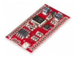
The MiniGen was designed to be used either as a stand-alone board or as a shield that can be placed on top of an Arduino Pro Mini. It's capable of generating sine, square, or triangle waves at up to 3MHz, and approximately 1Vp-p. The output is at a DC offset of Vcc/2. Neither the offset nor the amplitude can be varied.
