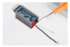
You can see a couple of points: the pin headers on the MiniGen have been soldered in with the long pins on the opposite side from the components, and the receptacles are on the component side of the Pro Mini.
