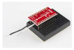
Flipping the board over, component side up, will allow you to mount it on a Pro Mini board that has female headers on its top side. I'll show you both of these cases fully assembled, so you can see the implications of each.
