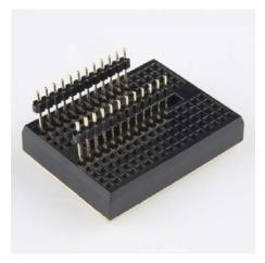
Once the pin headers are in place, you can lower the MiniGen board onto them. The board can be soldered on component side up or component side down; depending on what you plan to do with it, one of those is likely to be better.
