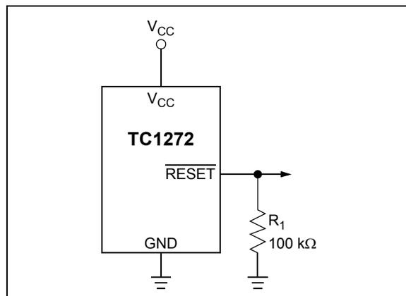
**FIGURE 4-6:** Ensuring Reset Valid To  $V_{CC} = 0\text{V}$ .
