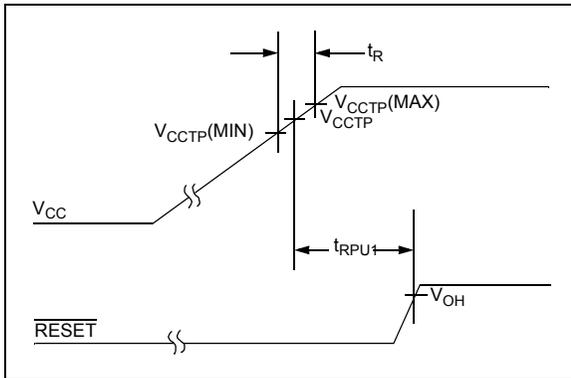
**FIGURE 4-1:** Timing Diagram – Power Up (TC1272/TC1273).
