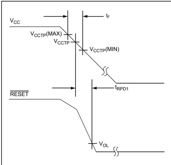
**FIGURE 4-2:** Timing Diagram – Power Down (TC1272/TC1273).
