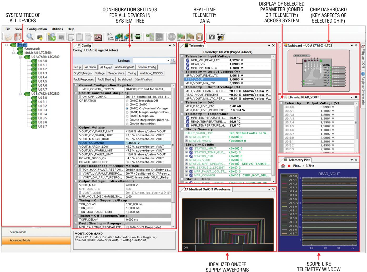
Figure 1. Screen Shot of the LTpowerPlay GUI
