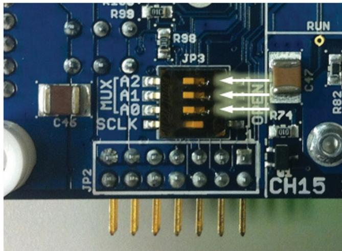
Figure 13. DIP Switch Set to All Zeros (0x20)
