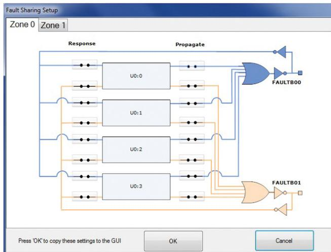
Figure 10. Fault Sharing Utility in LTpowerPlay GUI
