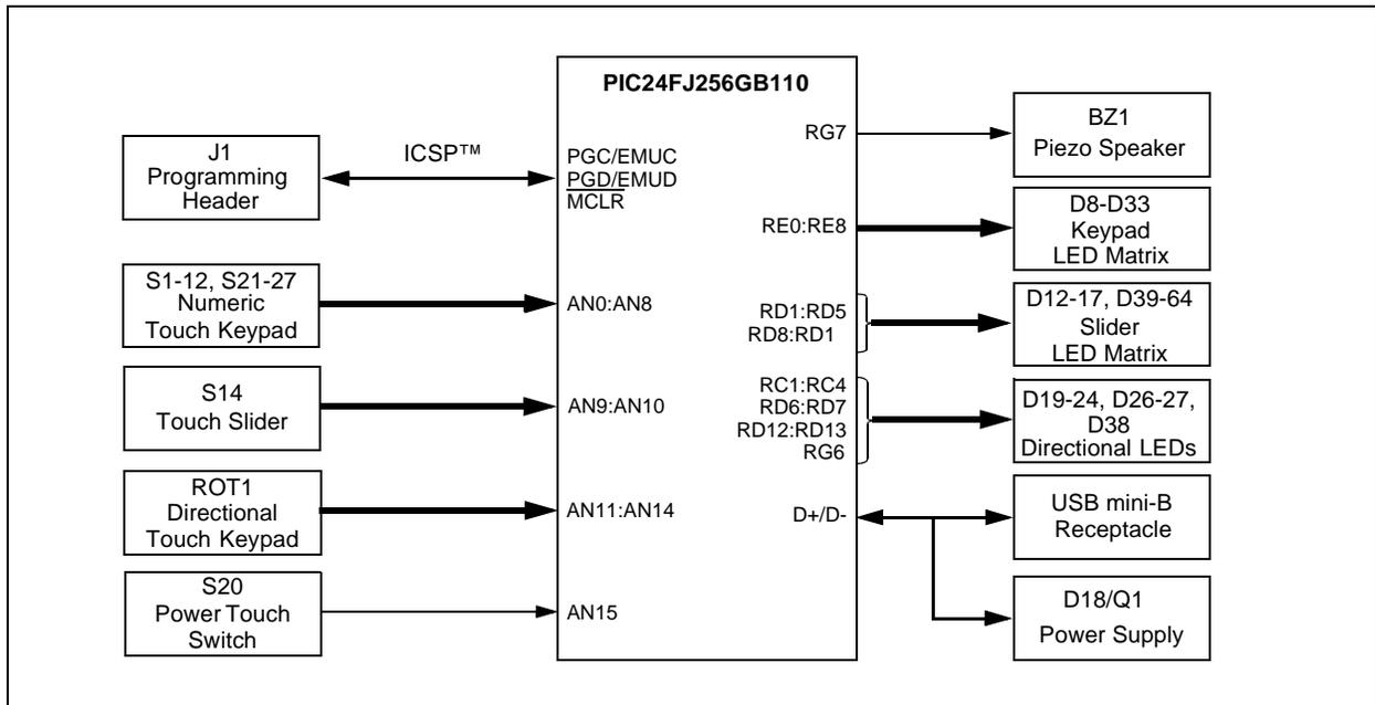
The operation of the demo board is managed by the PIC24FJ256GB110 microcontroller, which requires very little additional hardware to perform its tasks. In addition to the Touch Sense demo application code, the preloaded demo uses substantial parts of the Microchip USB Stack Library to provide a hardware interface to the PC-based interface application.
