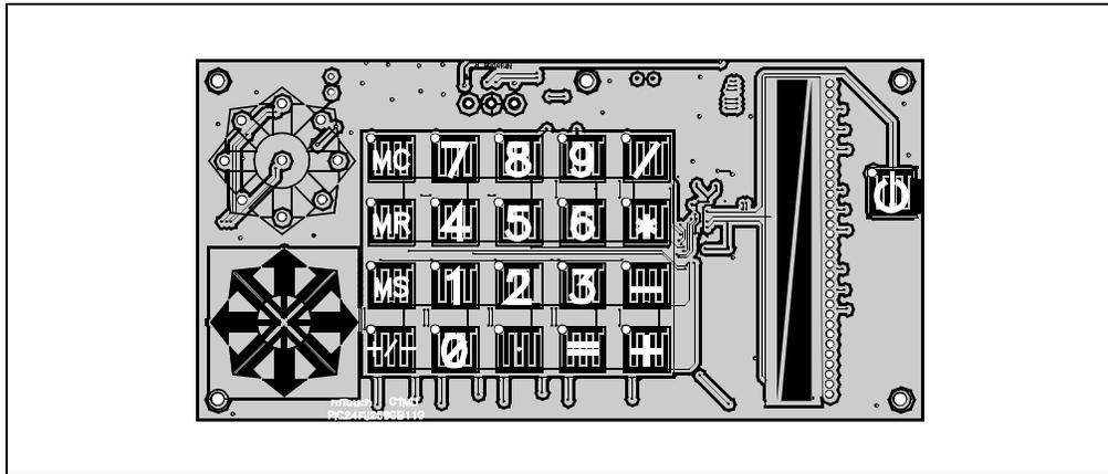
Nine of the A/D channels are used to monitor the numeric keypad switches (S1 through S12 and S21 through S27), arranged in a 4x5 array. Each “switch” is composed of interleaved conductors from two channels. The location of the touched key is determined by a simultaneous capacitance change on any two channels.
