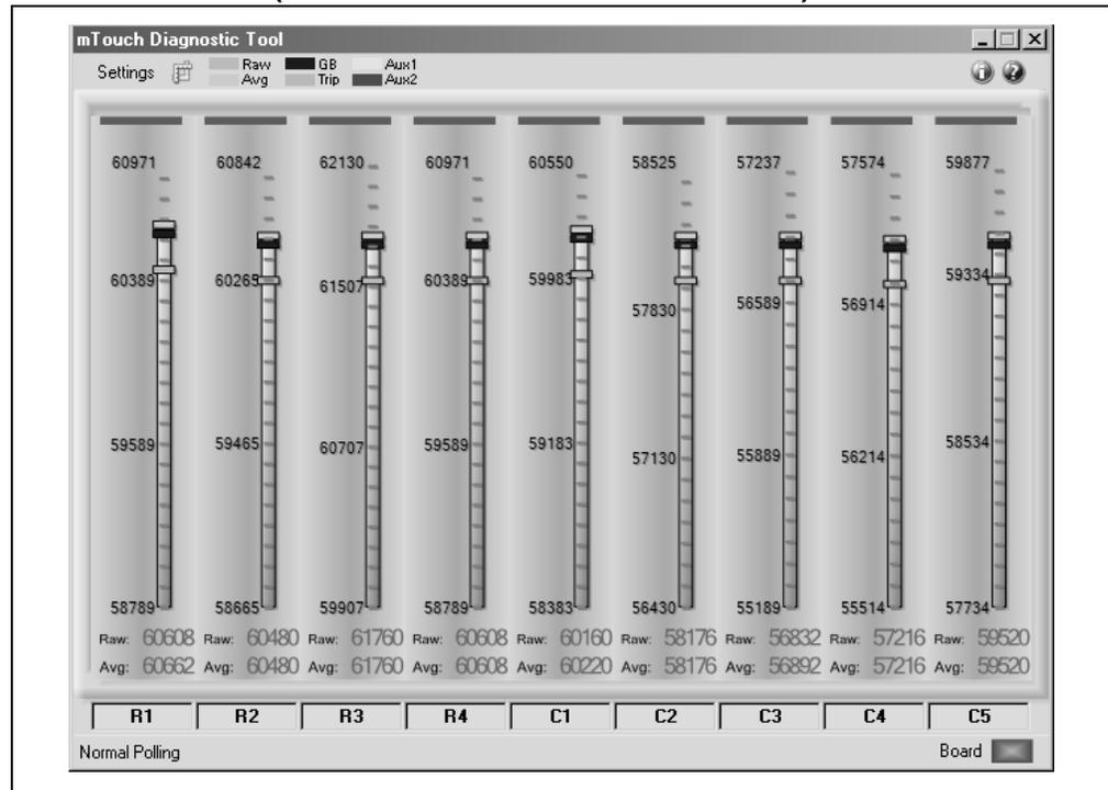
The A/D converter produces values of up to 1023 (10 bits). The PICDEM Touch Sense 2 Demo Board contains software algorithms that use scaled values of the raw A/D reading to improve averaging and overall performance of the hardware.
