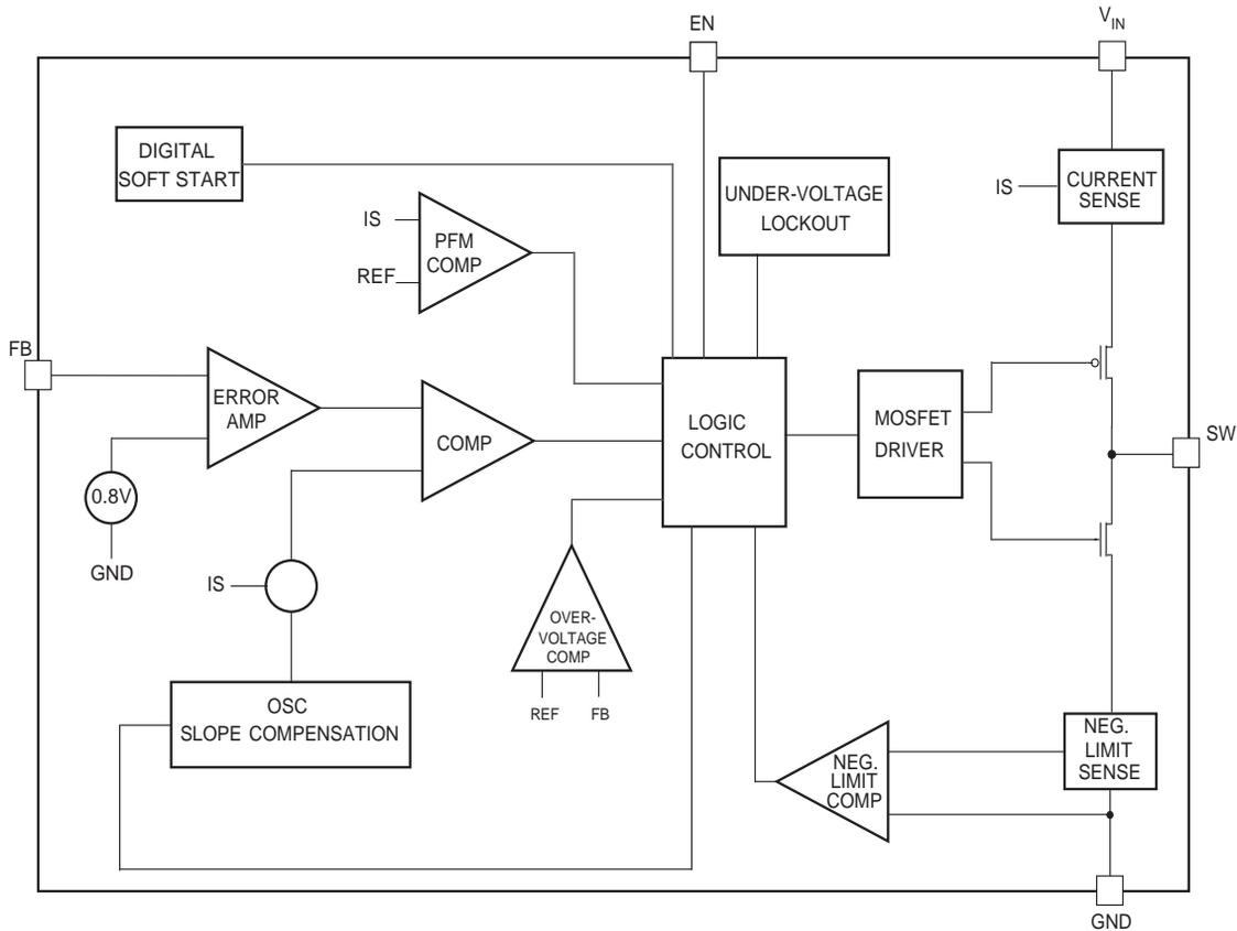
Figure 15. Block Diagram
