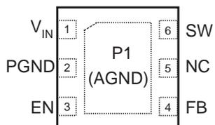
Figure 2. Pin Assignment for 3x3mm 6-Lead MLP
