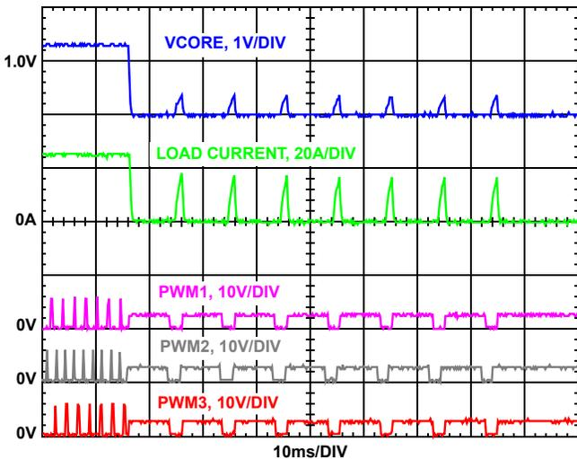
FIGURE 5. OVERCURRENT PROTECTION
