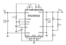
The EN2360Ql is a member of the Enpirion\* PowerSoC 12V DC-DC step-down converter family. When combined with the 5V and 6V step-down converters, designers of telecommunications, enterprise, storage systems, and industrial and embedded computing equipment have the broadest choice of integrated power management solutions for optimizing footprint and reliability in point-of-load applications without compromising efficiency, noise, or thermals.
