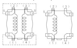
(3.3  $\mu$  H $\sim$ 15  $\mu$  H) (22  $\mu$  H $\sim$ 100  $\mu$  H) "S" is winding start.
