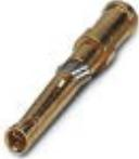
Turned 1.6 crimp contact, individual female contact, core diameter 0.75 to 1.00 mm<sup>2</sup>, gold-plated
