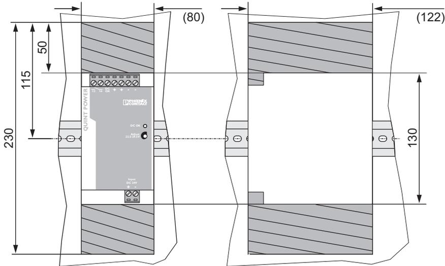
Slim-style installation: Installation depth 125 mm (+ DIN rail) (state at delivery)
