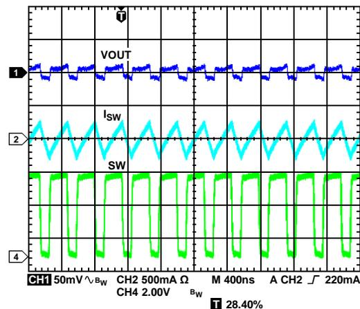
Figure 6. Typical Waveforms, V<sub>OUT1</sub> = 3.3 V, I<sub>OUT1</sub> = 30 mA, PWM Mode
