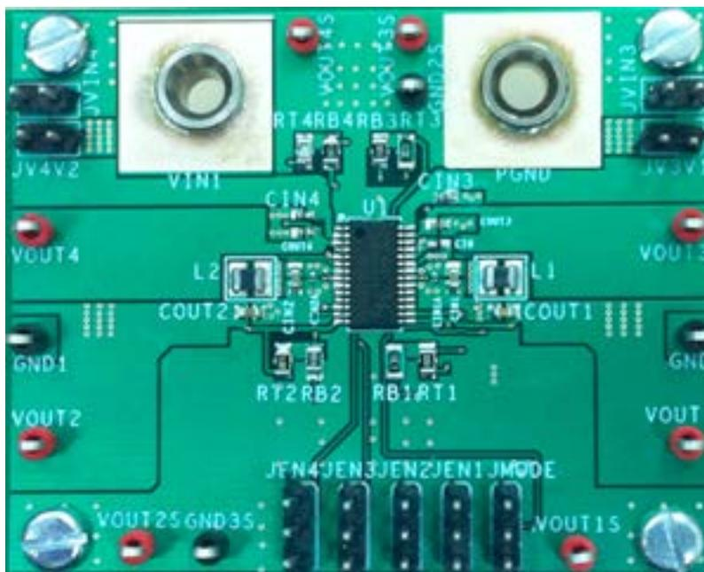
Figure 1. [ADP5034](#) TSSOP Evaluation Board
