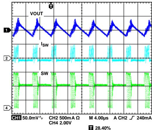
Figure 5. Typical Waveforms, V<sub>OUT1</sub> = 3.3 V, I<sub>OUT1</sub> = 30 mA, PSM Mode
