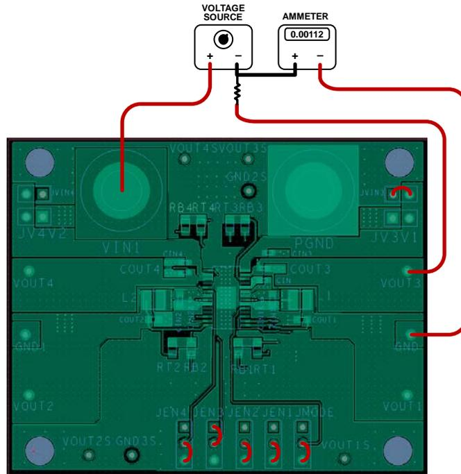
Figure 14. Ground Current Measurement
