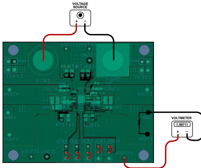
Figure 13. Output Voltage Measurement
