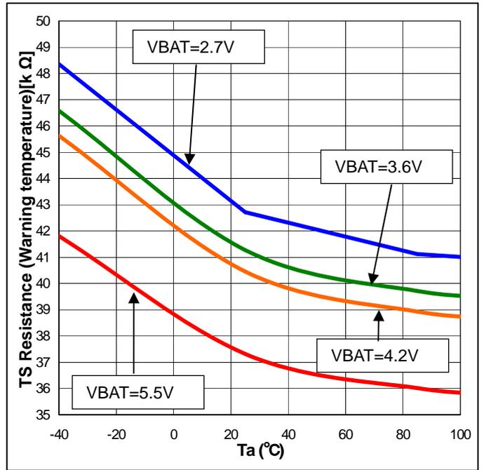
Figure 5-12. TS Resistance (Warning temperature) - Temperature
