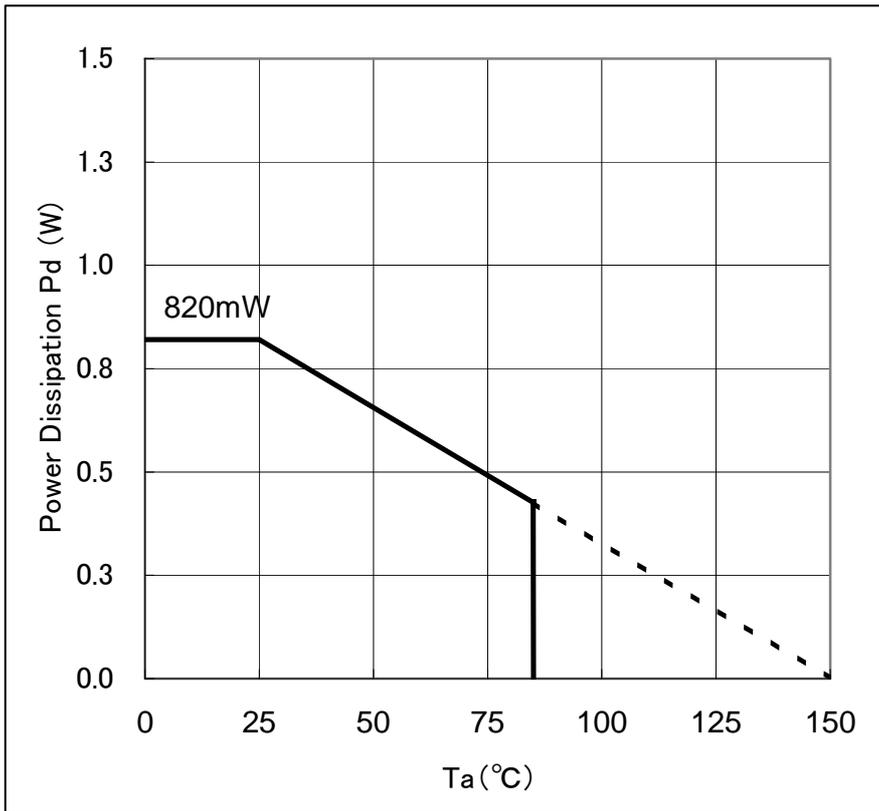
Figure 33. Power dissipation
