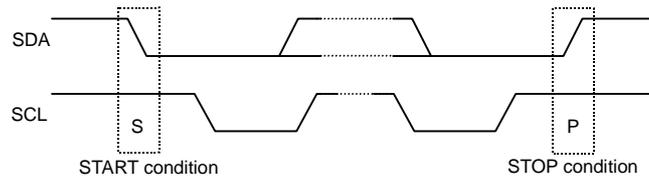
Figure 7. START/STOP condition (I<sup>2</sup>C format)
