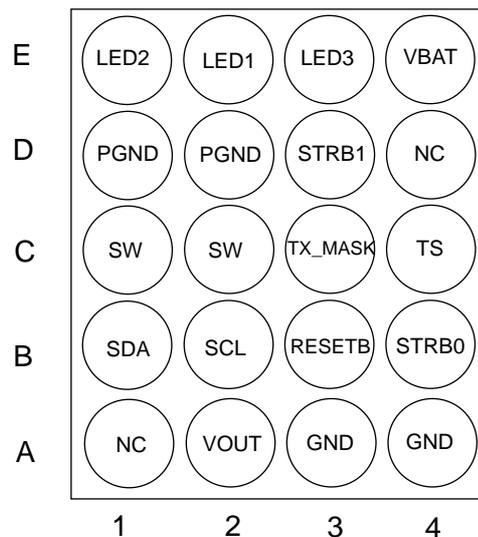
Figure 2. Pin Configuration
