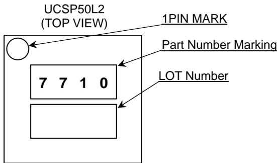
Figure 35. Marking Diagram
