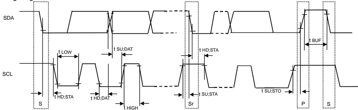
Figure 12. Timing diagram (I<sup>2</sup>C format)
