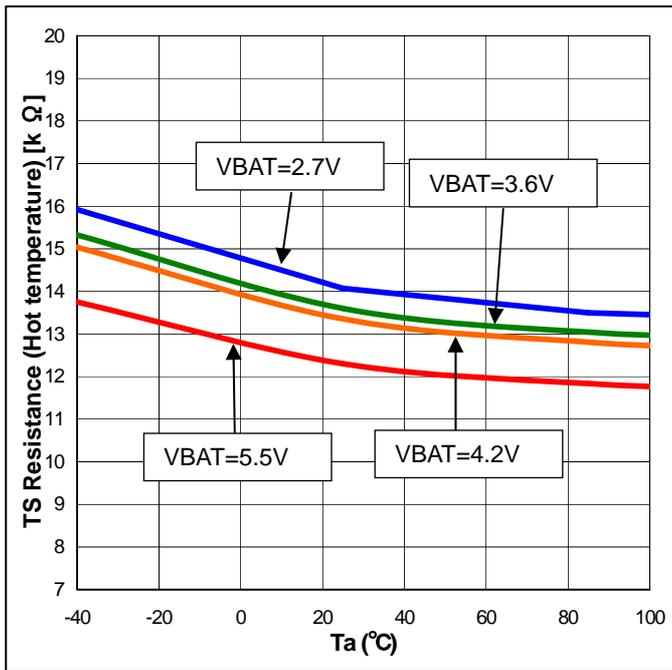
Figure 5-13. TS Resistance (Hot temperature) – Temperature
