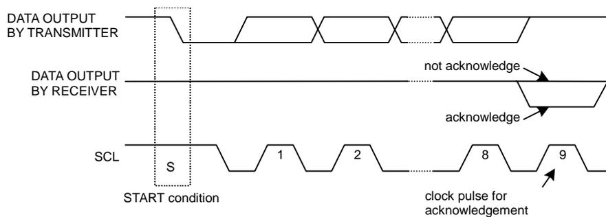
Figure 8. Acknowledge (I<sup>2</sup>C format)
