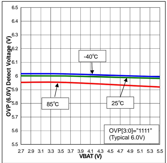
Figure 5-8. Over Voltage Protection (OVP) - VBAT
