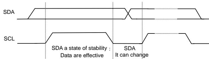
Figure 6. Bit transfer (I<sup>2</sup>C format)
