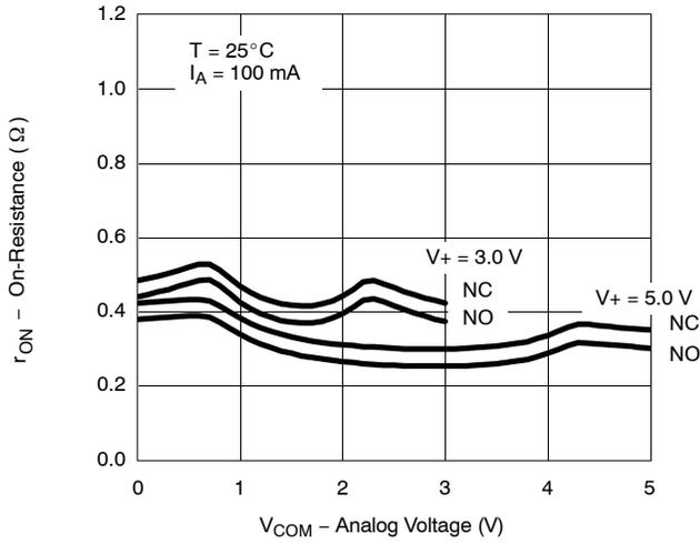
**r<sub>ON</sub> vs. Analog Voltage and Temperature (NC1)**
