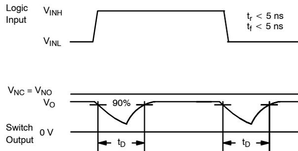
FIGURE 3. Break-Before-Make Interval
