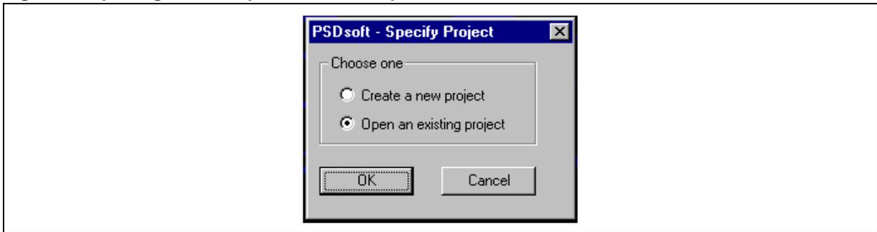
Use cancel at this point since all we need to do is program the PSD with an existing demonstration file (\*.obj) and there is no need to create a new project. Later, in the “Using the DK4000 as a development platform”, a further tutorial is given on using PSDsoft Express with the Eval Board for development.
