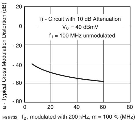
Fig. 3 - Typ. Cross Modulation Distortion vs. Frequency  $f_2$
